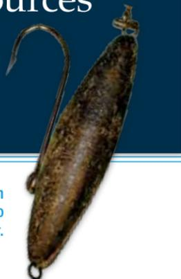
This fish descending device is constructed from an inverted barbless hook with a weight used to "escort" a bloated fish back to deeper water.
